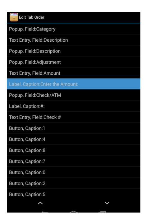
To adjust the tab order, select Adjust Tab Order from the Tools button. Here you will see a list of all the controls on the form. You can press the Up and Down icons to re-order as necessary.
